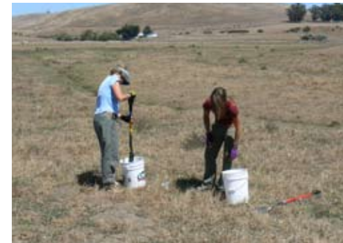
Photo 6, mix soil sub-samples in a bucket to prepare sample to send to the lab.
